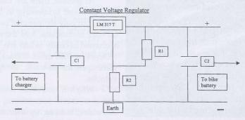
ICI LM 317T Voltage Regulator R1 240 ohms, .25 watt R2 5K potentiometer C1 0.1 mfd 150 volt C2 1 mfd 40 volt C1/C2 not critical Adjust R2 for 13.5 volts
